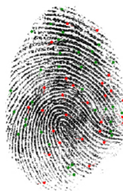
Fig.1: Image depicting what an ievo reader scans and key minutiae features.
